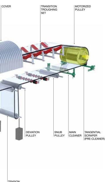
TENSION PULLEY WITH COUNTERWEIGHT
