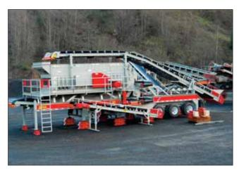
Driving cross belts, screen feeds, recirc belts, hopper feeders, transfer conveyors, and belts under screens and crushers, Rulmeca Motorized Pulleys are used on crushing/screening plants, stackable conveyors, radial stackers, reversing shuttle conveyors, and miniature conveyors in aggregate and frac sand production, highway construction, mining, and recycling.
