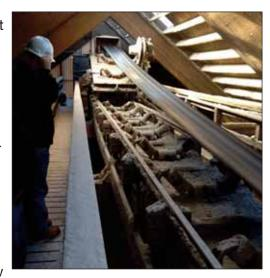
stainless steel 20 HP model 400M Motorized Pulleys in the head and tail positions.
