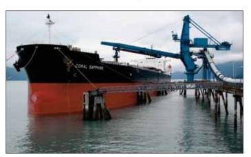
This Alaskan rail-to-ship transfer terminal installed a 75 HP 24.8" diameter Motorized Pulley in the ship loader shuttling boom conveyor when they upgraded the machine to handle 2,000 tph of coal. Faced with frigid conditions, the operator chose the optional anti-condensation heater, which maintains a constant warm temperature within the pulley shell when the machine is idle. Other operators use "trickle voltage" heating to serve the same purpose.
